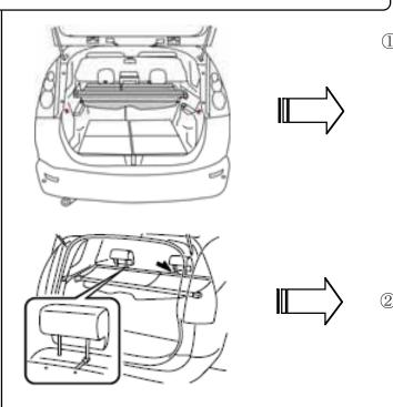
① Insert the holder into the concavity.
